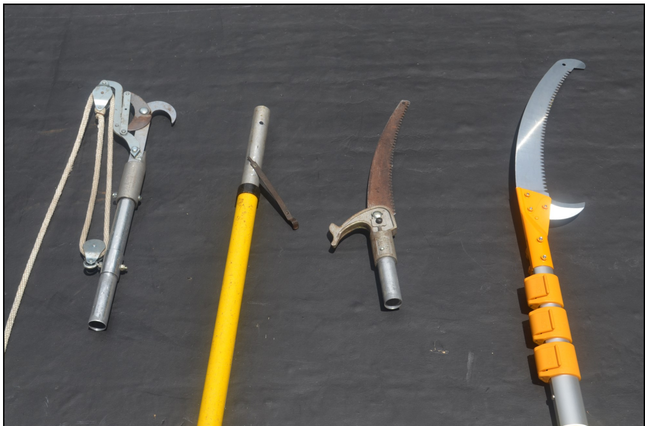
LEFT TO RIGHT: Bypass pruner; 12' telescoping pole with "leaf spring/pin" attachment; pole saw head with hanging hook; and 20' long aluminum telescoping pole with locking pins and toggle clamps
